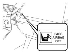
If the front passenger weight sensors are working properly, the indicator light illuminates when the ignition switch is turned to the ON position. After a specified period of time it goes out.
